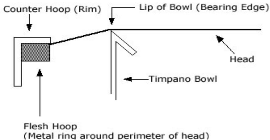
The best way to determine the correct size head you need is to take the head off the drum and measure the outside diameter of the head. Outside diameter means from one side of the metal ring to the other. If the head is still on the drum, you can measure from inside one tension rod across to the opposite tension rod:
